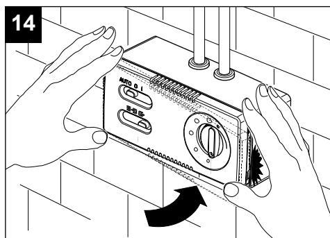
Note: it can be flush-mounted on containers with a pitch of 130 mm and a depth of 50 mm
