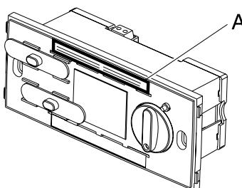
The power-source data must be consistent with the electrical data shown on the nameplate (A).
