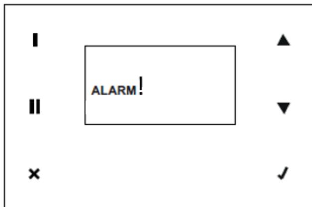
After 3 months if the filters are not replaced the unit will give a Filt alarm and stop operation until the filters are replaced and the message cleared as above.
